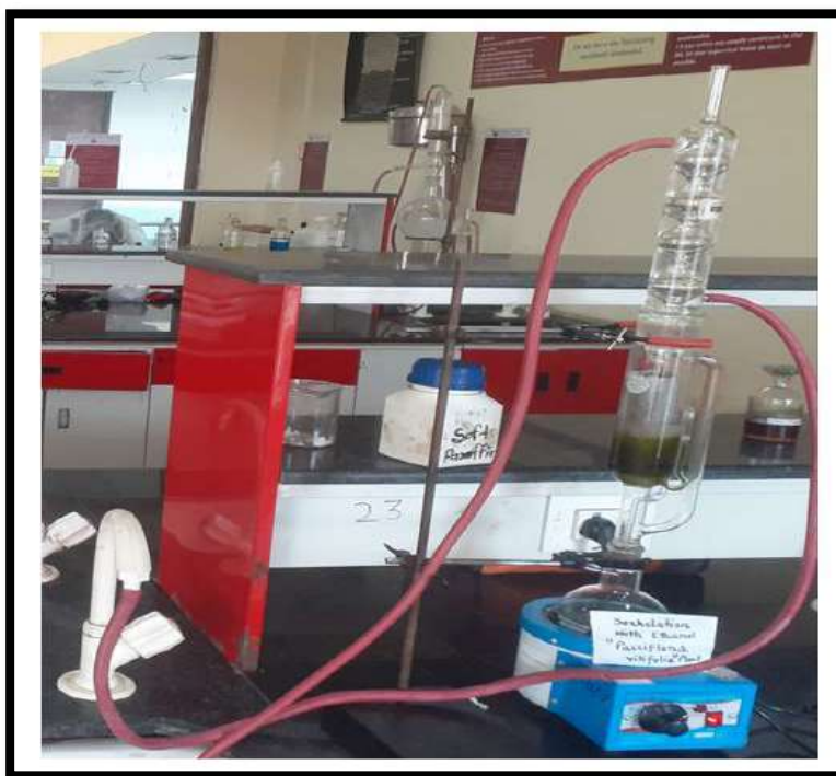
Fig 1.10: Representation of Soxhlation of ethanolic leaves extract of Passiflora vitifolia
