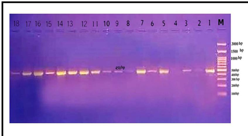
**Figure 7.** Gel electrophoresis of conventional PCR, the *Hms* gene from biofilm *S. marcescens* was amplified and then electrophoresis. Agarose 1.5%, 80 V/cm for 45 min, ethidium bromide dye staining, and UV transilluminator visualization. M: Marker ladder (100 -3000 bp). Lane (1–18)
