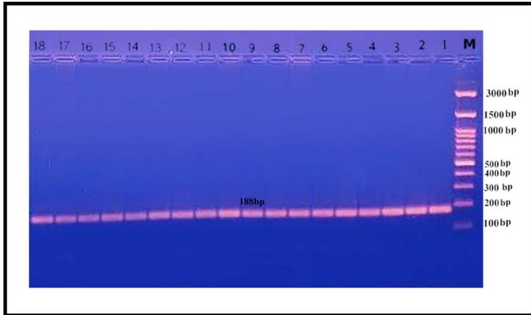
**Figure 6.** Gel electrophoresis of conventional PCR, the *SsmE* gene from Efflux pump *Serratia marcescens* was amplified and then electrophoresis. Agarose 1.5%, 80 V/cm for 45 min, ethidium bromide dye staining, and UV transilluminator visualization. M: Marker ladder (100 -3000 bp). Lane (1–18)
